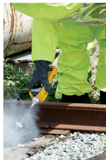
Workers can quickly measure VOCs and wirelessly transmit data via Bluetooth or optional Mesh radio.
